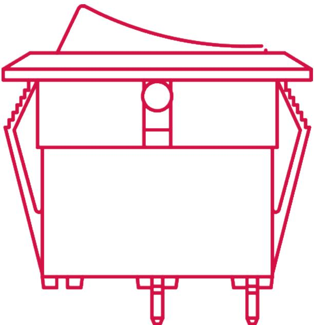
Rocker switches are commonly used as an on/off switch that rocks (rather than trips) when pressed, meaning the rocker opens or closes the circuit. This means that one side of the Rocker switch is raised while the other side is depressed, much like a seesaw or rocking horse.
