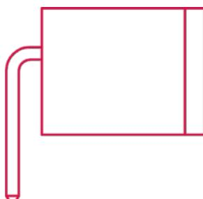
**Tilt switches:** Detect changes in orientation and then trigger actions, like making or breaking a connection, in response.
