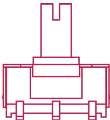
Rotary Switches use a rotating mechanism to select one of several positions. E-Switch products can feature up to four poles and 12 positions, and there are many actuator style and length options to choose from, as well as thru hole and solder lug termination styles.
