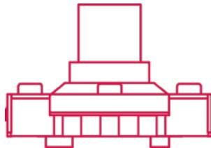
**Navigation switches:** Used for navigating through menus, options or interfaces on devices.
