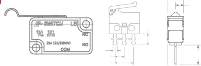
Snap Action switches, also called microswitches, are switch devices that can open and/or close an electrical circuit at a rapid speed. Triggered by an external force, either human or physical object, which is then applied to an actuator that requires very little pressure to operate.
