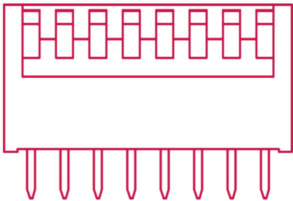
DIP switch refers to a set of electrical switches packaged in a small box or housing, which are arranged in a line or circle (rotary DIP). The function is to provide a range of electrical inputs to an electronic device based on the position of the individual switches within the line or circle. The main advantage of a DIP switch is the ability to quickly change positions.
