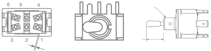
The Toggle switch is characterized by the presence of a manually operated handle or lever which controls the flow of electrical current from power supply to device, such as a household appliance.
