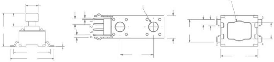
Tactile, a.k.a Tact, switches are used to close an electrical circuit when pressed. When the switch is released, it opens the circuit.
