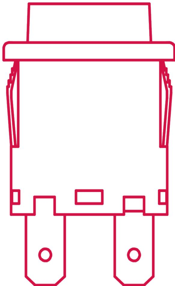
Pushbutton switches open or close an electrical circuit by pressing or, in some cases, pulling on the actuator. Deciding on the size, style and functionality of the pushbutton is often determined by the application.
